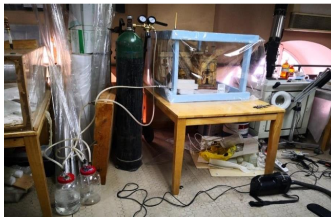
Fig.10. Showing Fumigation process using Carbon dioxide with tent
