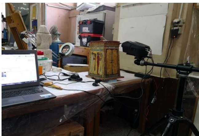
Fig.1. Showing identification of Egyptian pigments by X-ray florescence (XRF)
