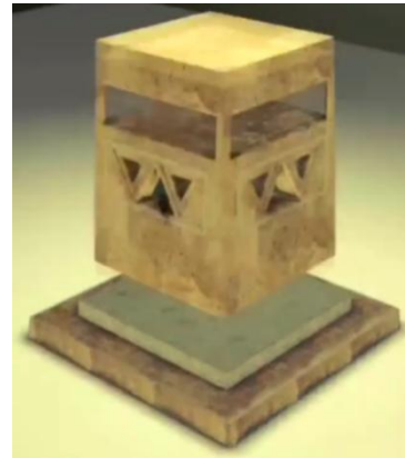
Fig 4. General perspective of the components of al-saqqāyāt in Ḥaḍramūt showing the base and the water chamber. Source: Ḥaḍramūt Center for Historical Studies, Documentation, and Publication.
