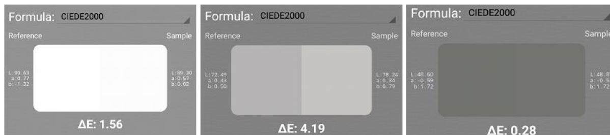
Fig. 12. \Delta E^* values and visual representation of the color change resulting from storage of photographic samples in sample (LN) post artificial aging. Highlights (left), midtones (center) and shadows (right).
